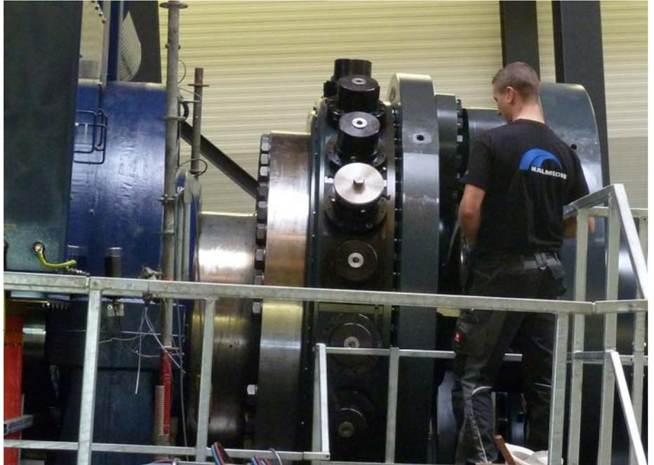
With an astonishing shut-off torque of **12.100.000 Nm**, the coupling is equipped with 21 Safety-Elements ASE40.
